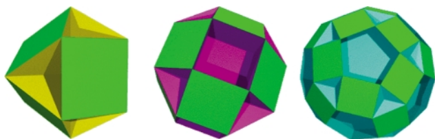
Fig. 1 The three types of faceted uniform polyhedra that can be generated by linking the vertices of squares only: cubohemioctahedron , small rhombihexahedron and small rhombidodecahedron .
