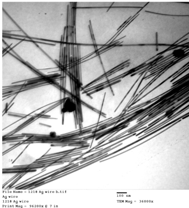
Fig. 2 TEM image of shape-separated silver nanowires; scale bar = 100 nm.
