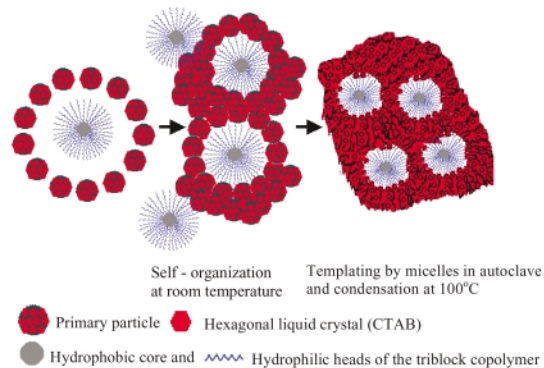
Fig. 3 Schematic representation of bimodal pore formation in the second step.
